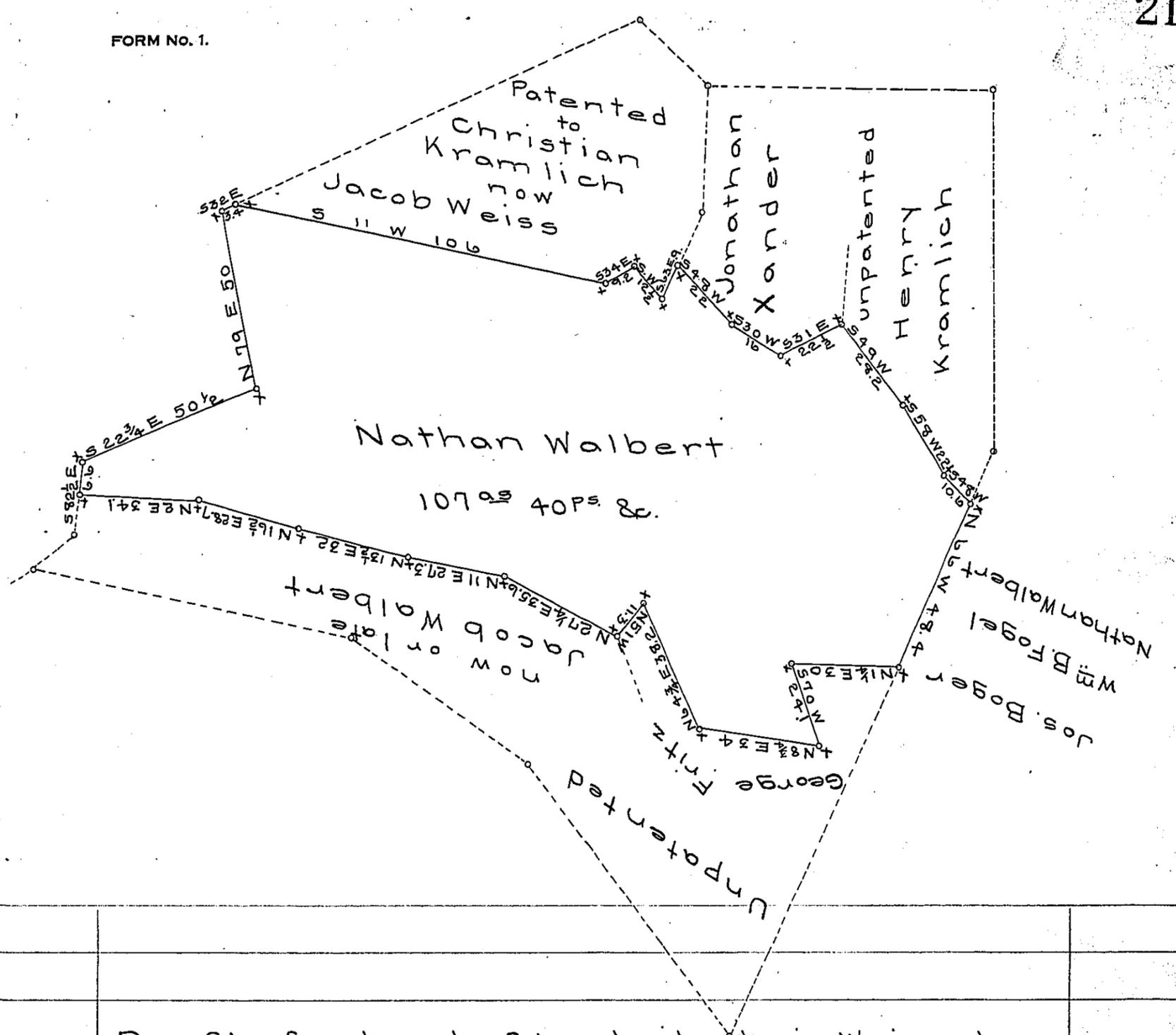
Draft of a tract of land situate in Weisenberg township, Lehigh County containing 107<sup>ac</sup> 40<sup>ps</sup> and allowance of six per cent for roads &. Being a part of a larger tract of 225<sup>ac</sup> and allowance originally surveyed in pursuance of a warrant granted to Ludwig Riffel dated the 29<sup>th</sup> day of Jan'y A.D. 1753. The above portion thereof now returned for Nathan Walbert
